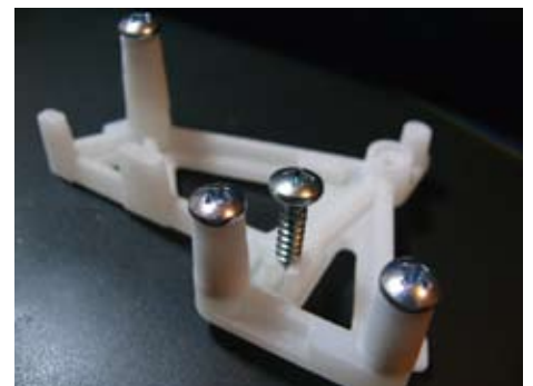
DuraForm® PP100 Plastic can be used for self-tapping screws.
