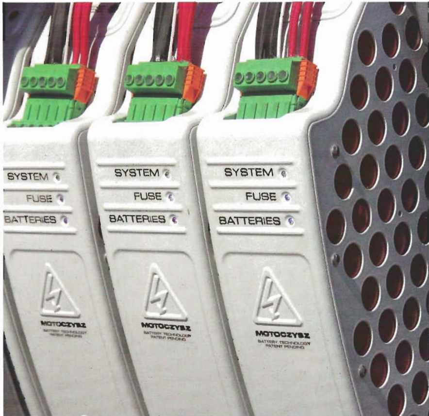
“Hot-swappable” battery packs incorporate LED lighting that indicates battery-management system integrity, fuse status and battery life at a glance.
