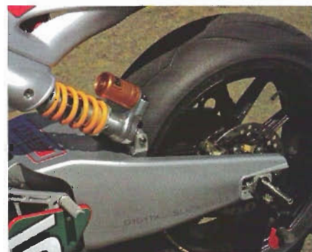
A unique, pushrod-activated rocker mechanism allows Czynsz to quickly and easily alter ride height and rear suspension progressivity.
