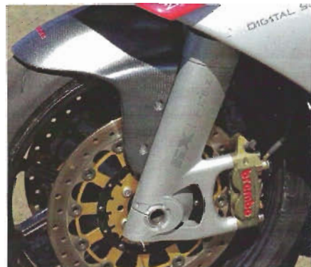
The 6X Flex fork is an all-new, tuned-flex design. “It was a bit of a job,” Czynsz says, “but we wanted the latest spec, not the same old C1 fork.”
